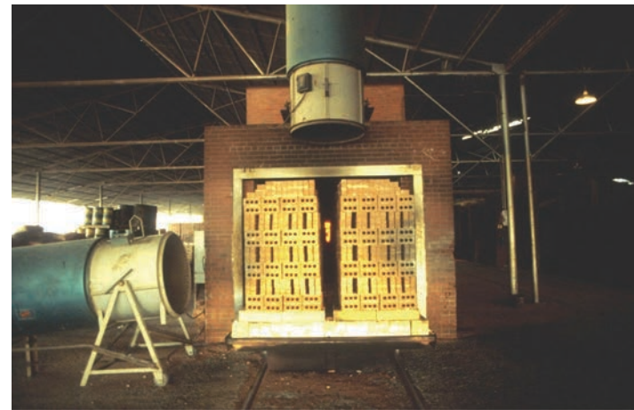
stiff mud manufacturing process tunnel kiln
