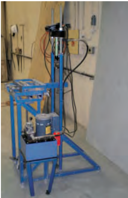
Fig. 2-5 ASTM C1072 bond wrench apparatus. (IMG25759)
