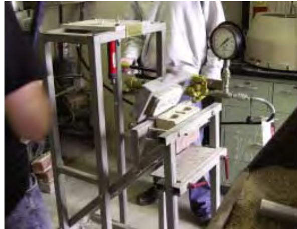
Fig. 2-6 The C 1072 bond wrench test being run. (IMG24170)
