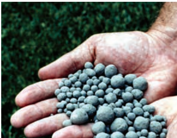
Fig. I-5 Pelletized aggregate made from fly ash and cement. (IMG15667)
