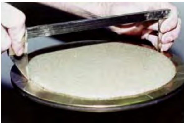
Fig. 2-8 Flow test. (IMG14093)
