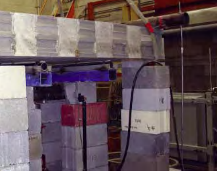
Above: A fully grouted masonry panel being prepared for flexural strength testing. See Fig. 3-3 for the panel in a deflected (loaded) condition. Photo courtesy of the National Concrete Masonry Association. (IMG24885) Right: Loads acting on masonry walls are described as axial, shear, and lateral loads. See Fig. 3-8.
