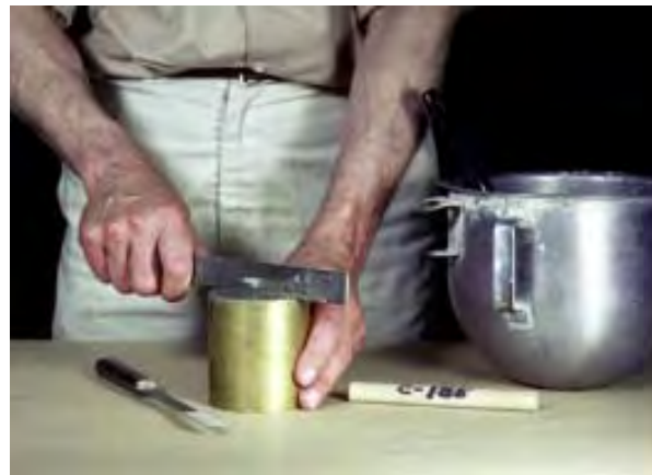
Fig. 2-9 Air content test. (IMG15606)
