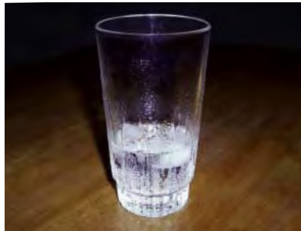
Fig. 3-18 Beads of water on the outside of this glass of ice water are caused by condensation of water vapor in the air as it comes in contact with the cold surface. (IMG24889)
